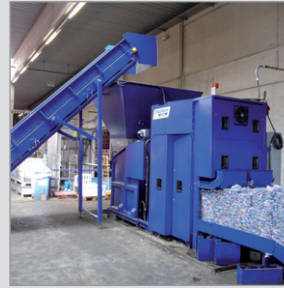
Filling by means of a conveyor belt
