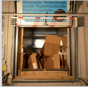
Feed opening through wall
