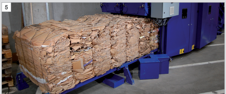
5 The finished bales can be stacked and are discharged fully automatically.
